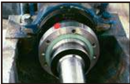
CVSD™ installed on a Slurry pump.
