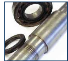
Shaft damage from a labyrinth seal
