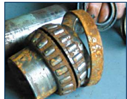
Moisture contaminated bearings
