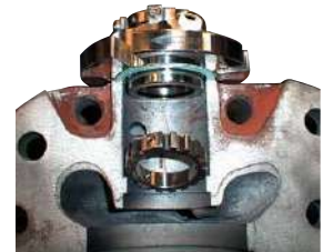
Separate conventional seal and pumping ring configuration.
