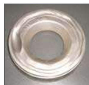
Effects of abrasion and erosion on a seal gland plate.
