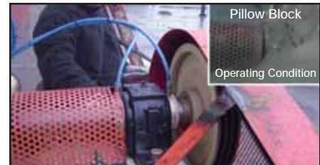
LabTecta-OAP-PB™ installed on a Pillow Block duty
