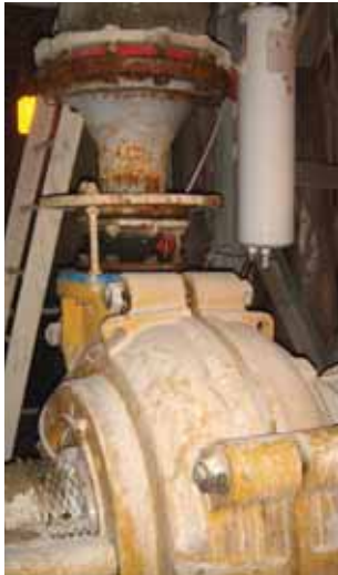
Double seal and SSE-25™ System installed on a Slurry pump
