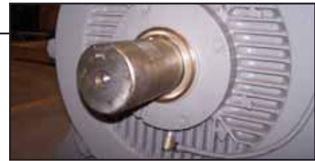
LabTecta™ installed on an Alumina Electric Motor duty
