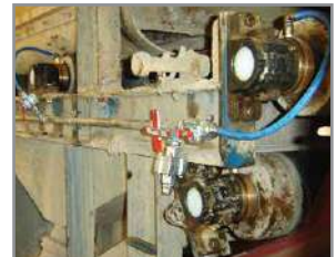
LabTecta-OAP-PB™ installed on mining conveyor belt
