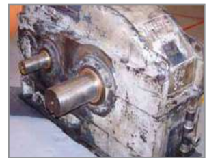
LabTecta® installed on a Falk gearbox
